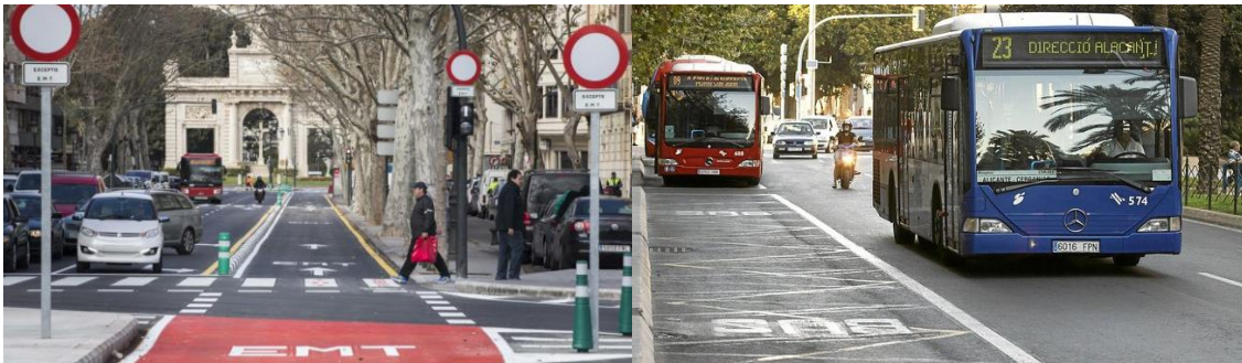
Figure 21; Left: contraflow bus lanes increase convenience of public transport [Photo of València (Spain) by German Caballero]. Right: Pull-Out Stops are just recommended in specific cases such as in timing points, with likely waiting times. Otherwise, buses lose time trying to steer back to the circulation [Photo in Alicante (Spain) by P. Rubio].
