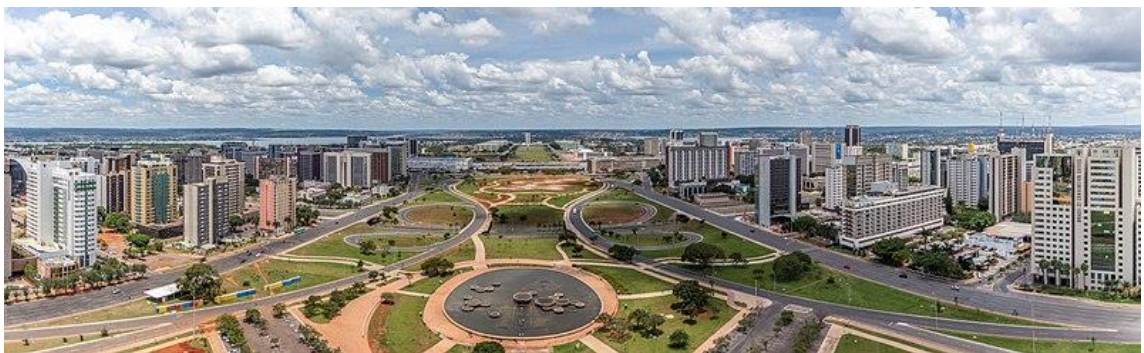
Figure 3; Perspective of the Eixo monumental, arterial road of Brasilia. It features the shape of a plane and all land uses are totally segregated and connected by a vast network of highways. Author: Webysther. Source: Wikipedia. Retrieved from: https://commons.wikimedia.org/wiki/File:Webysther_20180212132345_-_Esplanada.jpg
