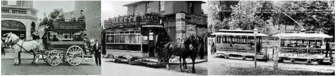
Figure 2; Omnibus, Horsecar and Tram. Source: "The History of Public Transportation". Retrieved from: https://infographic-journal.com/the-history-of-public-transportation/
