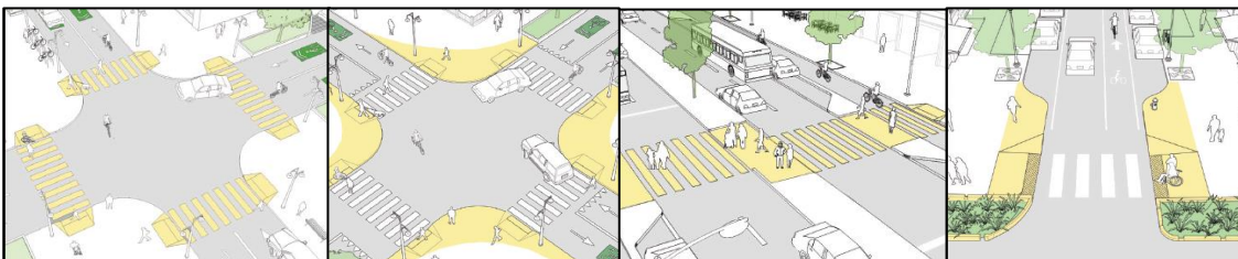
Figure 19; Different design techniques. Respectively: intersection design with 4 crossings; radii tightening; pedestrian refugees and bulbs-out, sidewalk extensions (Source: Global Street Design Guide, NACTO).
