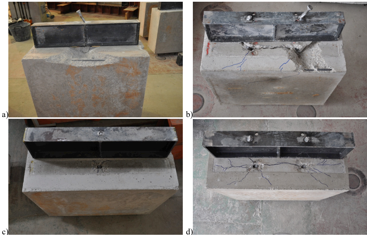
Figure 15. Specimens at peak load: a) specimen 1sM; b) specimen 2sM; c) specimen 1sC; d) specimen 2sC.
