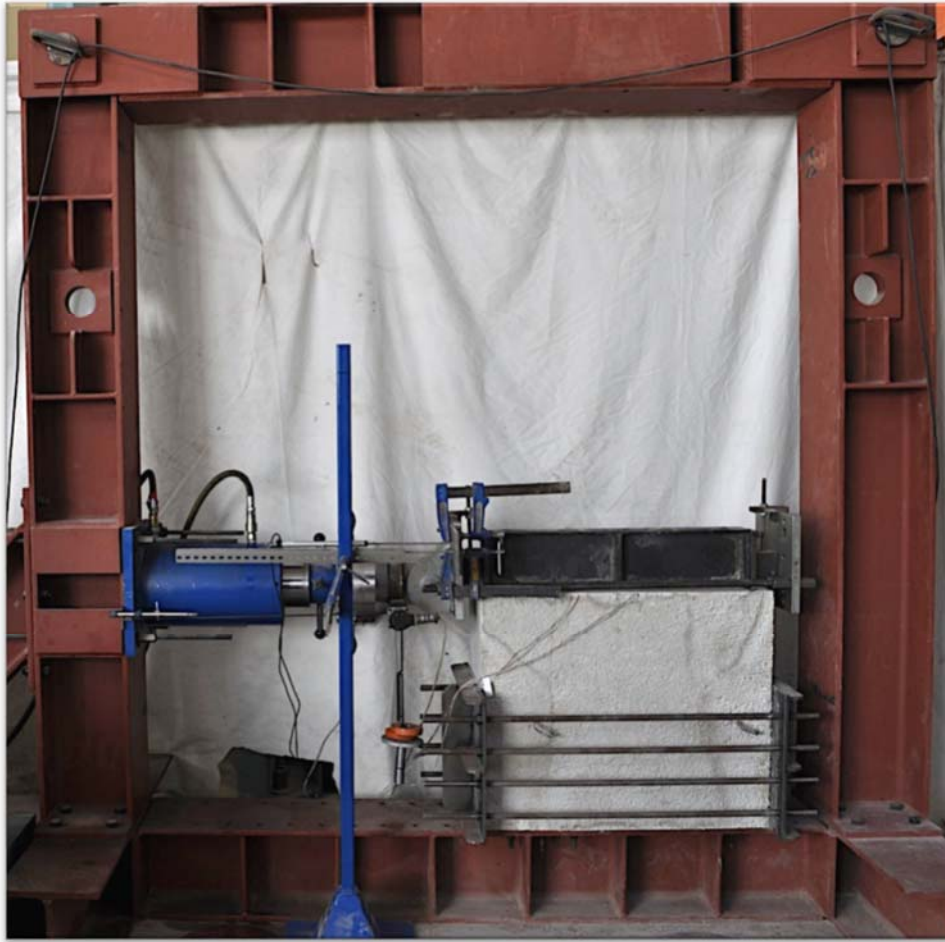
Figure 4. Test setup for headed studs in reinforced concrete panels subjected to shear forces.
