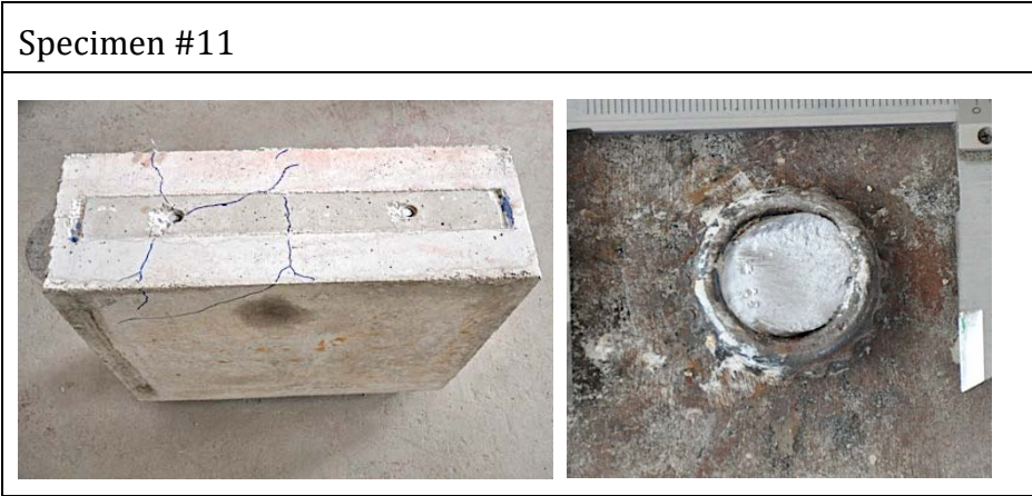
Figure 18. Steel failures on specimens for SRS configuration.
