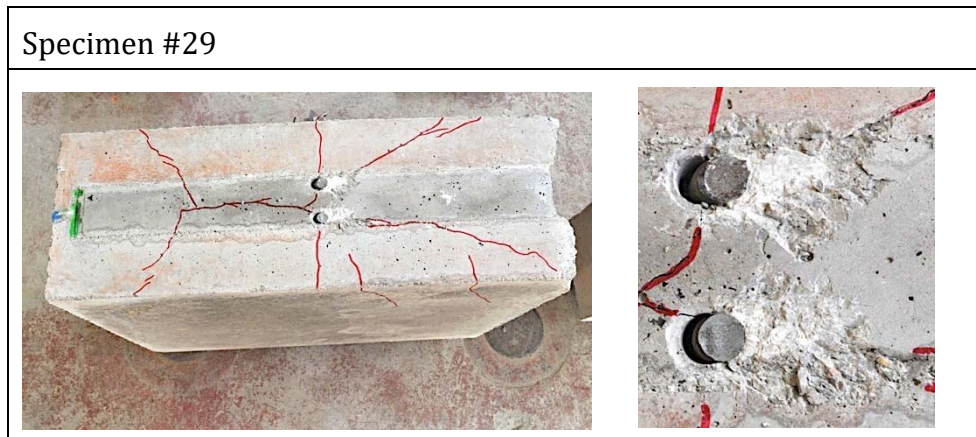
Figure 22. Steel failure in TRS-GE configuration.
