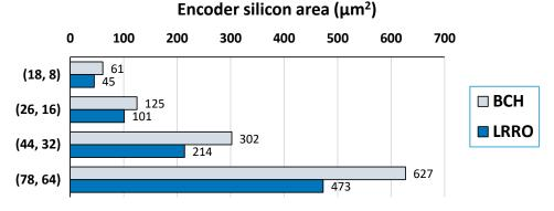
**Figure 9.** Silicon area occupied by the encoder circuits (in  $\mu$ m<sup>2</sup>).
