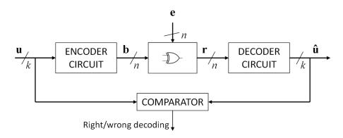
Figure 5. Block diagram of the error injector [21].
