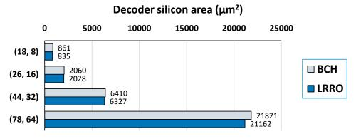
**Figure 10.** Silicon area occupied by the decoder circuits (in  $\mu m^2$ ).
