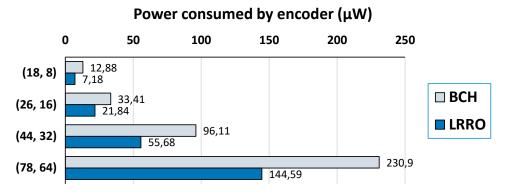
**Figure 11.** Power consumed by the encoder circuits (in  $\mu$ W).
