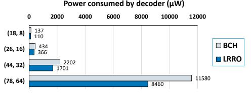
**Figure 12.** Power consumed by the decoder circuits (in  $\mu$ W).
