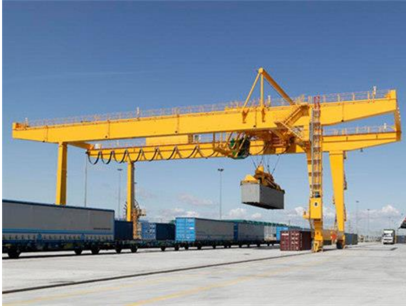
Figure 10. Gantry crane (AICRANE, 2020)
