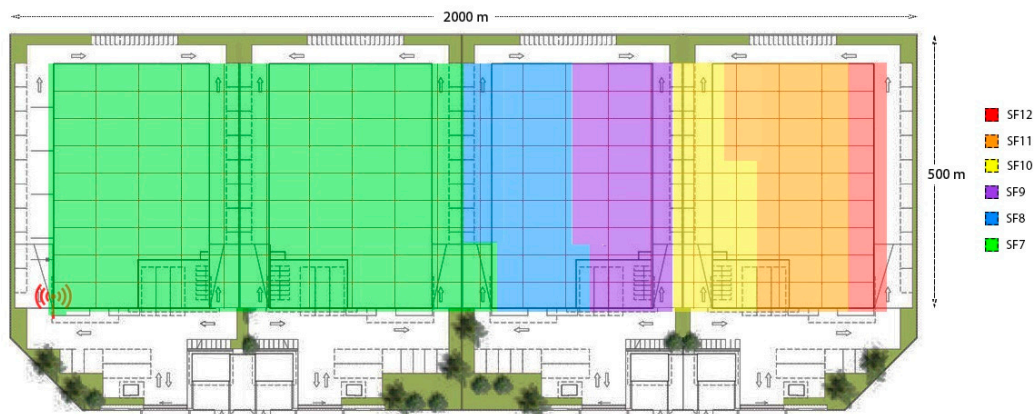
Figure 9. Results of SF for uplink traffic configured in every node at the end of the simulation, overlaid on the site map.
