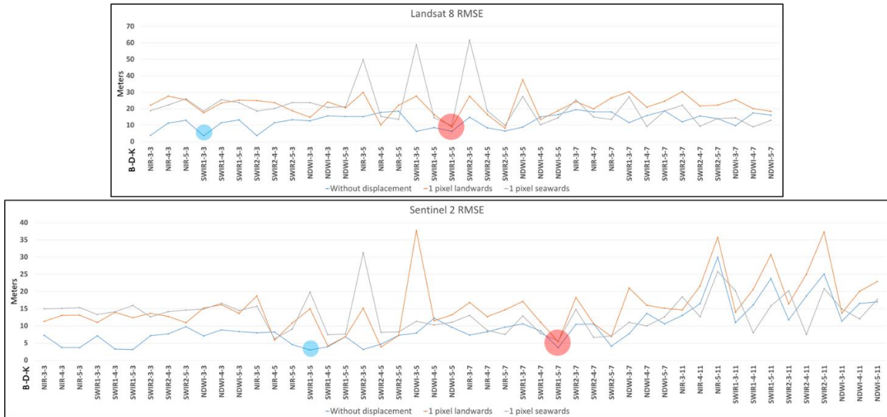
421 422 Fig. 11. Accuracy expressed in RMSE values for each combination of parameters in the x-axis (results of 423 Test 1 and 2). B-D-K initials mean: input Band, polynomial Degree and Kernel size. Red circles identify 424 the combination with best global behavior for all series despite the accuracy of the initial line, whereas 425 blue circles identify the best combination in absolute terms (best sub-pixel solution).
