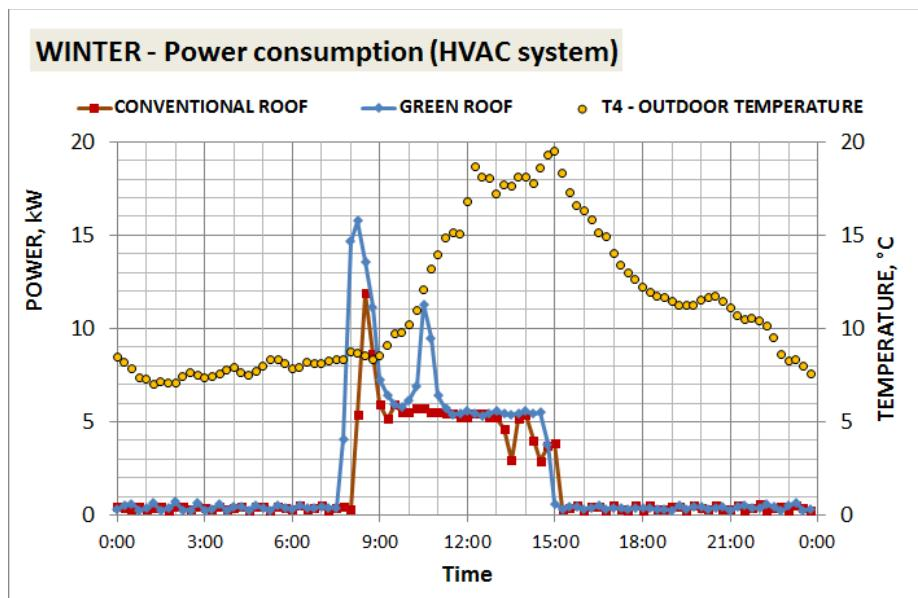
**Figure 12.** Comparison of similar days with and without a green roof in the winter period.
