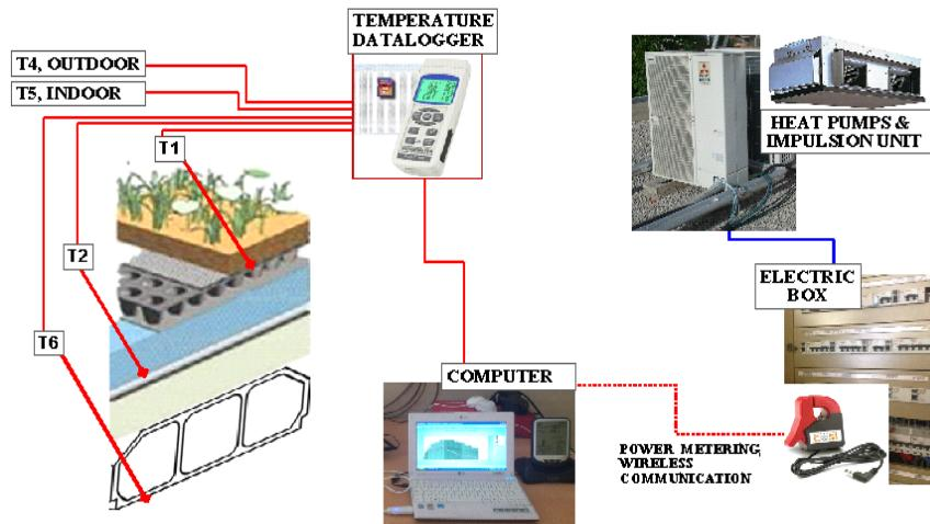
**Figure 7.** Monitoring system scheme.
