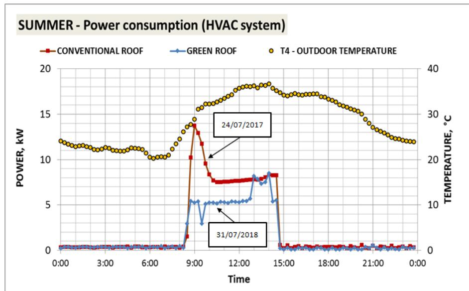
**Figure 11.** Comparison of similar days with and without a green roof in the summer period.
