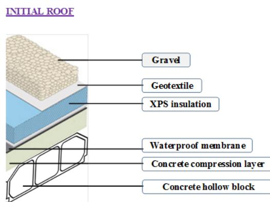
**Figure 3.** Initial roof structure.
