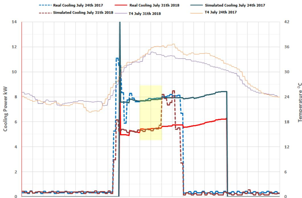
**Figure 15.** One-day validation of the models for conventional and green roof.
