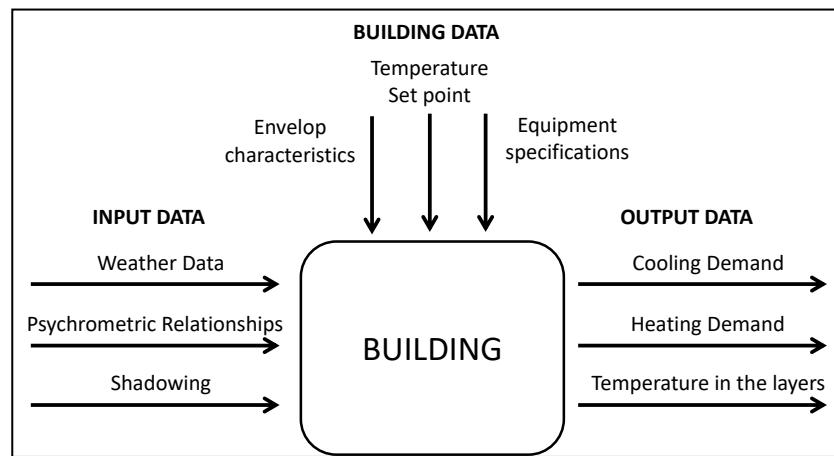
**Figure 13.** Parameters of TRNSYS Model.
