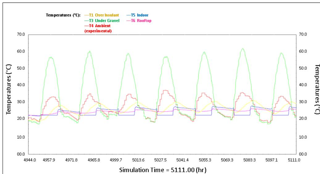
**Figure 14.** Simulated temperatures of the initial rooftop.
