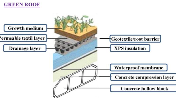
**Figure 4.** Green roof structure.
