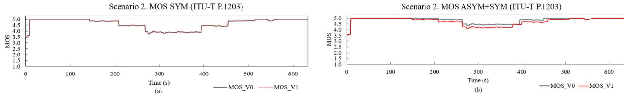
Figure 21. ITU-T P.1203 O.34 output for Scenario 2. (a) MOS per second using SYM representations. (b) MOS per second using ASYM+SYM representations.
