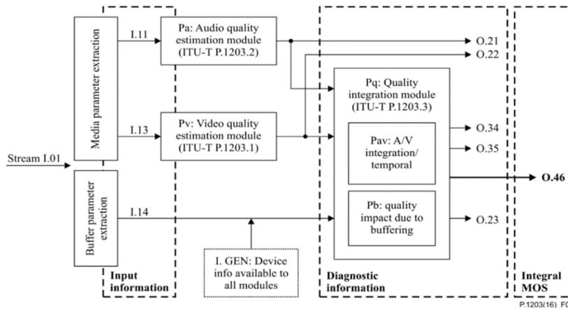
Figure 7. Model ITU-T P.1203 architecture overview.
