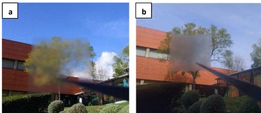
Figure 3. Background transparency pictures of the electrospun PHBV biopapers: (a) derived from MBW and (b) commercial grade.
