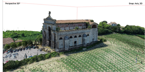
Figure 4: Final point cloud.
