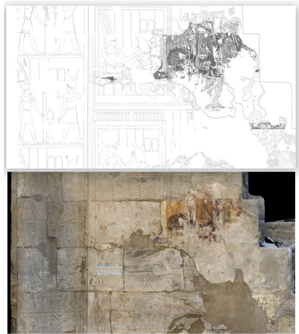
Figure 13: Drawing from Photogrammetry. Sample of drawing (top) from photogrammetric orthomosaic (bottom) on the south west wall, used for fresco documentation as well as inscribed AIII Pharaonic material behind. Vertés, Murray/The Epigraphic Survey 2017, 2018.
