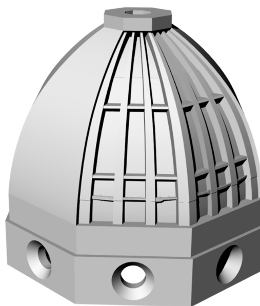
Figure 4: The 3D model of the dome of Santa Maria del Fiore inclusive of all its main construction elements.
