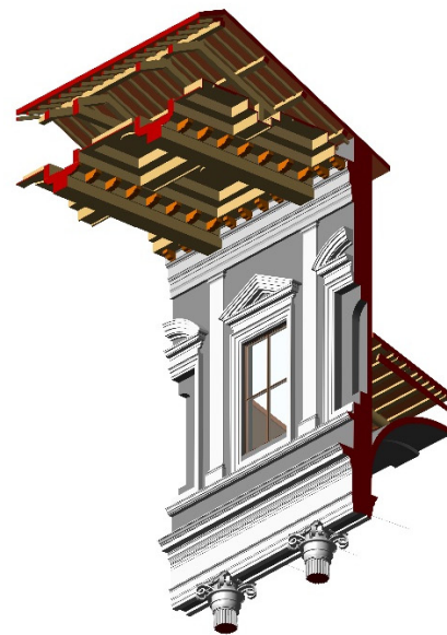
Figure 8: Cut-away axonometric views of the model with the ceiling components together: a) entire ceiling; b) detail of a portion.
