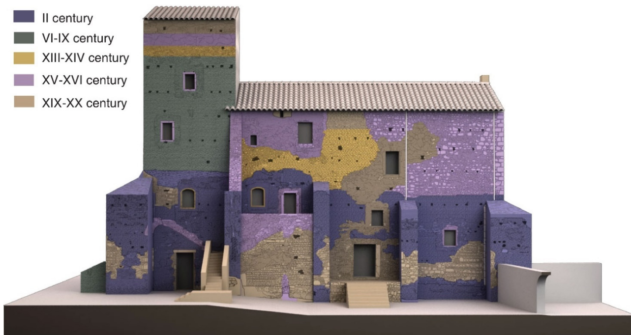
Figure 7: Stratigraphic analysis of the masonry on the 3D model of the Casale di Santa Maria Nova, southern façade.
