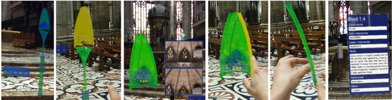
Figure 2: MR point cloud model interaction example. From the first low resolution point cloud it is possible to navigate through sequential increasing resolution point clouds reaching the 3D model of the marble block. Information could be attached at each step.
