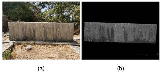
Figure 3: Ancient pedestal of the worshipping statue from the cella: a) visible-spectrum image; b) 3D classification of the surface weathering by texture segmentation.
