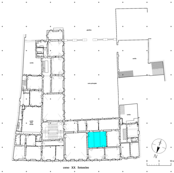
Figure 3: Main floor plan of Palazzo Magio. In cyan it's evidenced the floor with joists and planking renewed in the late 17 th -early 18 th centuries.
