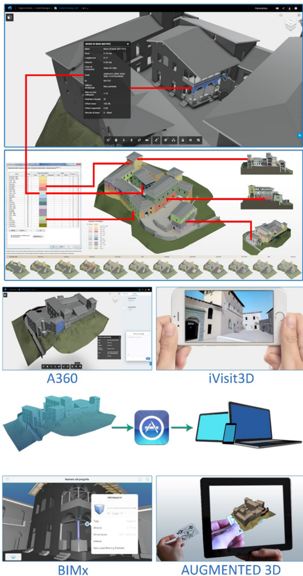
Figure 13: BIM model of the Castel Masegra depicting chronological phases of the building that was used for mobile VR and AR applications (Barazzetti & Banfi, 2017).
