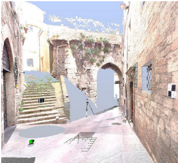
Figure 18: Coloured point cloud derived by a single scan.
