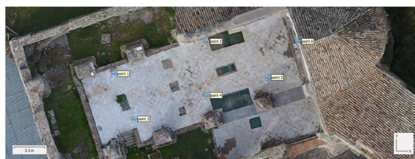
Figure 22: Ground control points materialized with the automatic RAD recognition target. November 2019.
