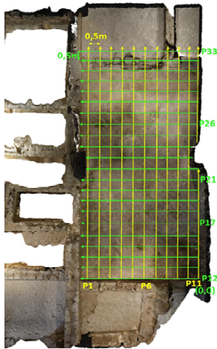
Figure 7: Layout of the GPR profiles in a grid 0.50x0.50 m (22 transversal and 11 longitudinal profiles) on the Roman pavement of opus caementicium of 3 rd century AD.
