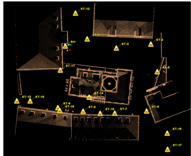
Figure 9: Distribution of simulated scan stations around the university office building.
