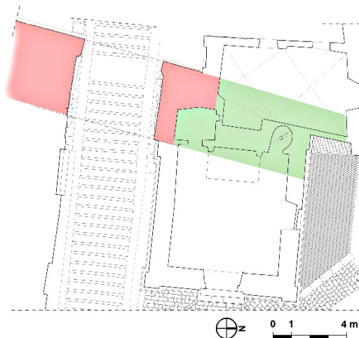
Figure 13: Plan of the gate and the adjacent Madonna dei Lumi church with highlighted the section of walls almost completely dismantled (green) to build the church.
