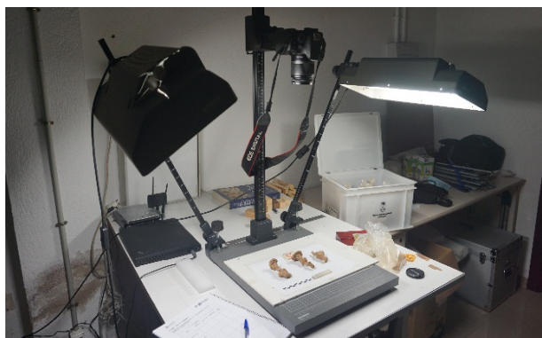
Figure 2: Photography process on a table type Kaiser® RS10 Copy Stand.
