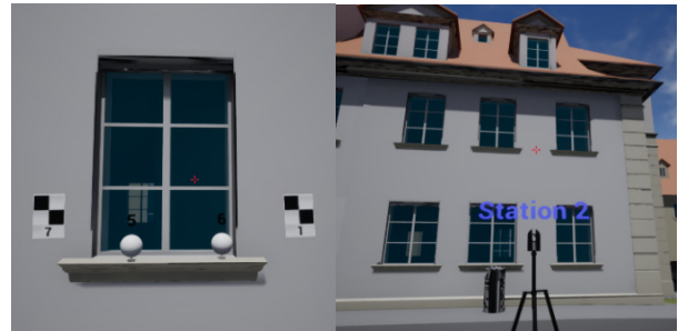
Figure 6: Target placing and laser scanner positioning in VirScan3D software around the university office building.
