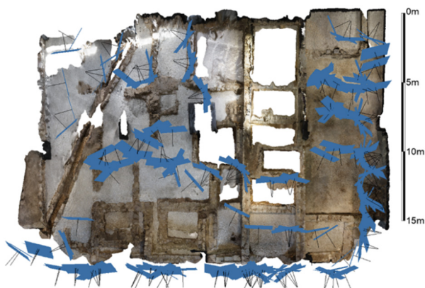
Figure 4: Distribution of each of the positions (blue) and orientations (black lines) of the photographic shots.
