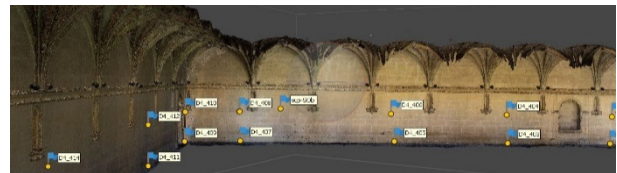
Figure 2: Half of the south elevation inside the cloister (dense point cloud with markers).
