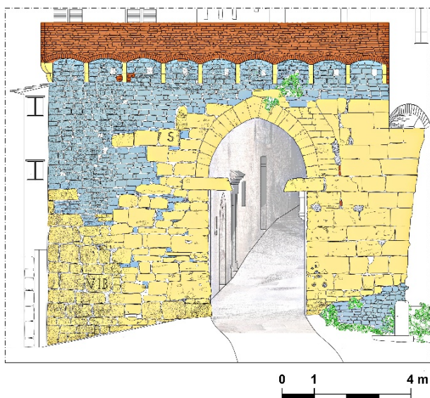
Figure 5: External front of the gate with highlighted the ashlars in travertine (yellow), limestone (blue) and the brick parts (red).
