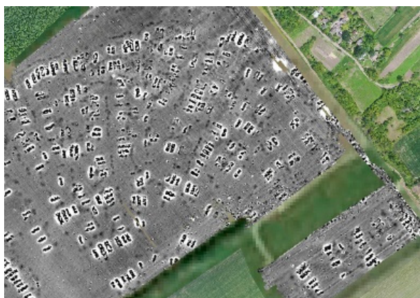
Figure 4: Orthophoto of the territory with superimposed geomagnetic survey.
