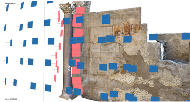
Figure 15: Corinthian Column Camera Positions. Screen shot of the camera positions used to photograph behind the column on the south west wall of the Imperial Cult Chamber. Murray/The Epigraphic Survey 2017.
