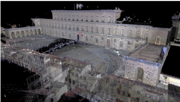
Figure 1: General view of the main façade of Pitti Palace (point cloud obtained by laser scanner survey).
