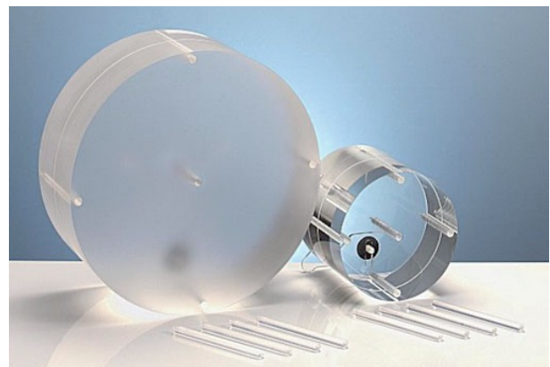
Figure 2: Cylindrical polymethylmethacrylate phantoms of 320 and 160 mm diameter with accommodations for the ionization chambers (Faggioni, Paolicchi, & Neri, 2010).
