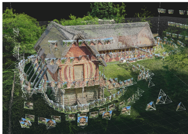
Figure 5: Camera positions and 3D model of the reconstructed Trypillya buildings.
