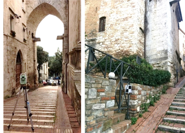
Figure 16: Total station survey, with checkerboard targets and reference spheres on the left.
