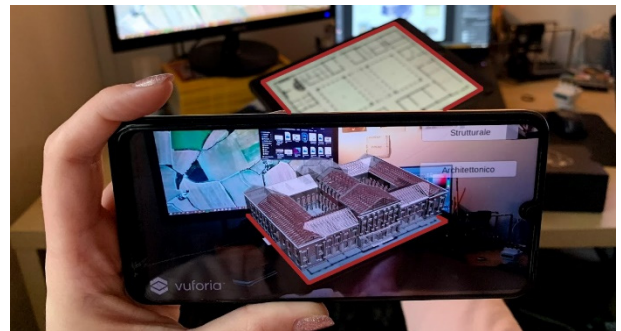
Figure 12: A view of the structural model through the AR app.
