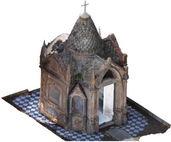
Figure 6: The mesh model produced with Agisoft Metashape.
