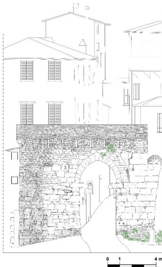
Figure 24: Example of CAD drawing (vertical section) obtained by a scan cutting plane.
