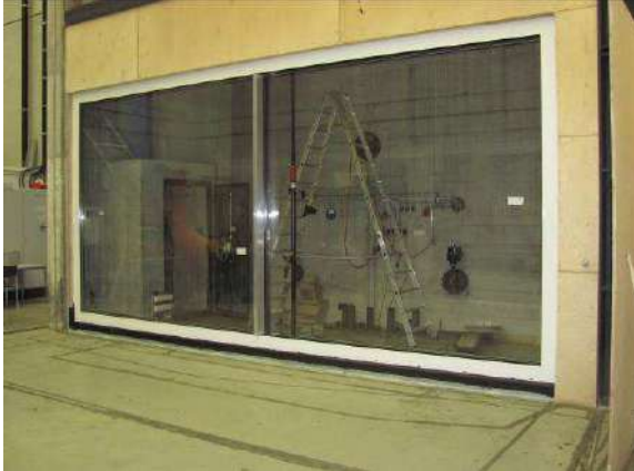
Photo 1 Test specimen on test rig, window closed
