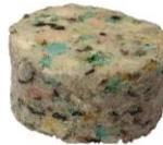
Figure 1. Recycled polyurethane foam used in this work.
