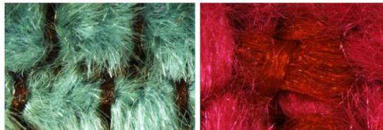
Figure 2. Surface and the warp/weft pathways of the textile materials is analyzed with microscope imaging technique with 16X magnifications. **left:** T1; **right:** T2.
