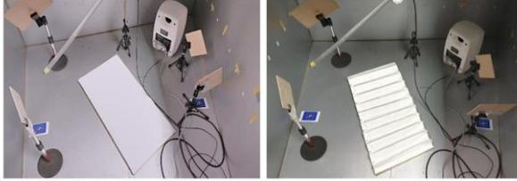
Figure 8. Experimental setup in the small-sized reverberation chamber. Fabric samples correspond to the configurations a) T0 and b) T8.
