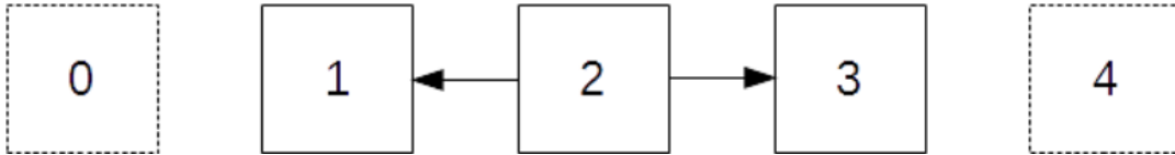
Figure 3.3: Communication pattern of LAMMPS in one of the dimensions.
