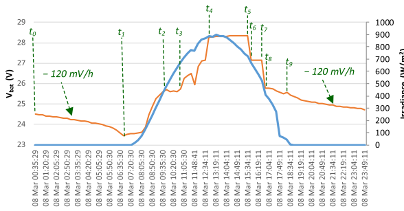
FIGURE 7. Voltage in the battery and irradiance during 8 March.
