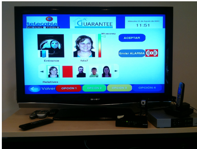
Figure 8.1: Picture of the set-up in the Guarantee Project: an interactive IPTV shows the results of face recognition (using HOG-EBGM) from a peep-hole camera at the main entrance of a home.
