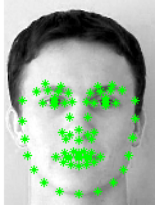
Figure 6.13: Real example of a face graph generated using the AAM model matching technique, with graph models of N_n = 58 landmarks.
