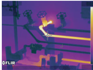
(e) Industry. Pump leak detection [12].
