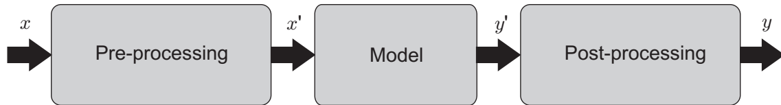
Figure 2.1: Block diagram of a modeling scheme that includes preprocessing and post-processing.
