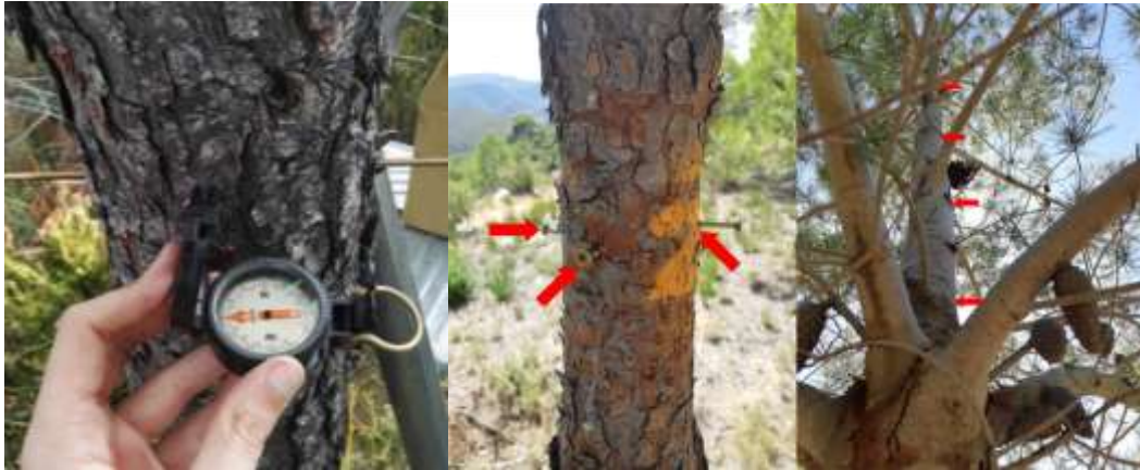
Figure 3 Electrode placement using a compass (left), identification of trees and radially location of the electrodes (centre), electrodes separated longitudinally (right).
