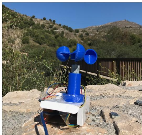
Figure 10. Node with the anemometer.
