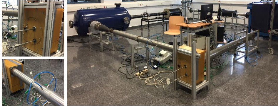
Figure 8. On the top left, the two pitot tubes. On the bottom left, the pressure and temperature sensors in the duct. On the right, the flow bench installation.
