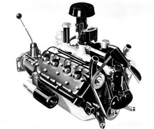
Figura 2.10: Motor Flathead V8 de 1932
