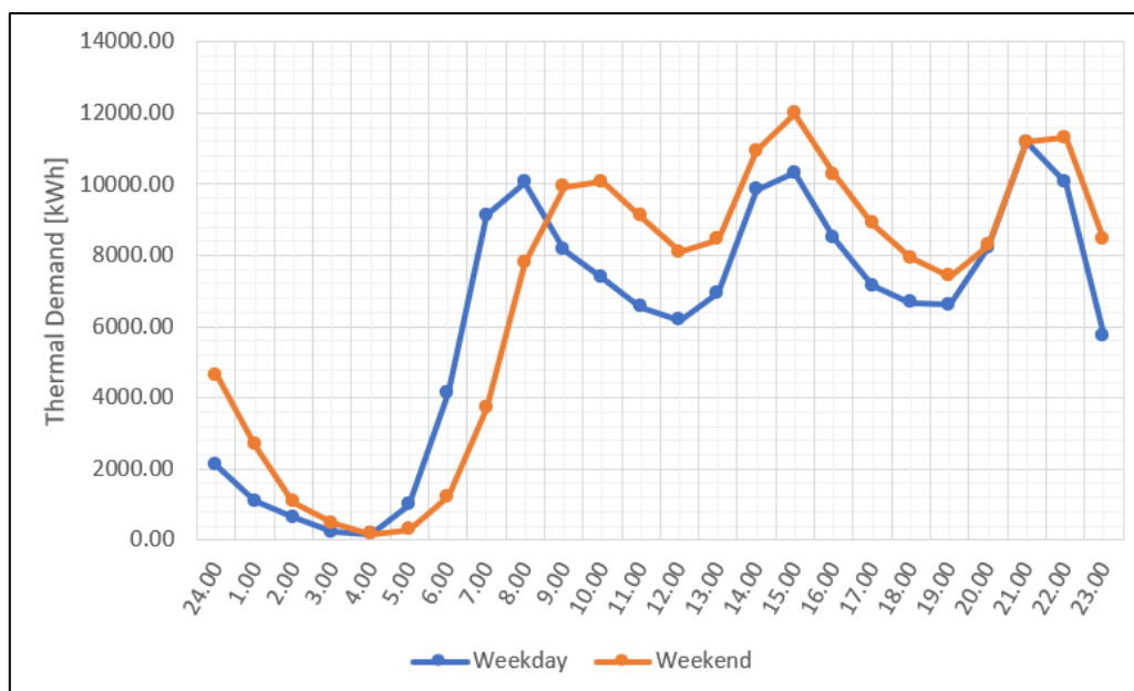
Figure 12 - Daily thermal demand curves for a typical weekday and weekend day in February
