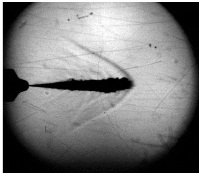
128 Figure 2. Example of shadowgraphy visualization image for test in sulfur hexafluoride environment.
