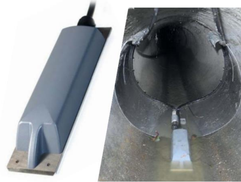
Figure 2. Ultrasonic flowmeter. Source: Mejoras energéticas
