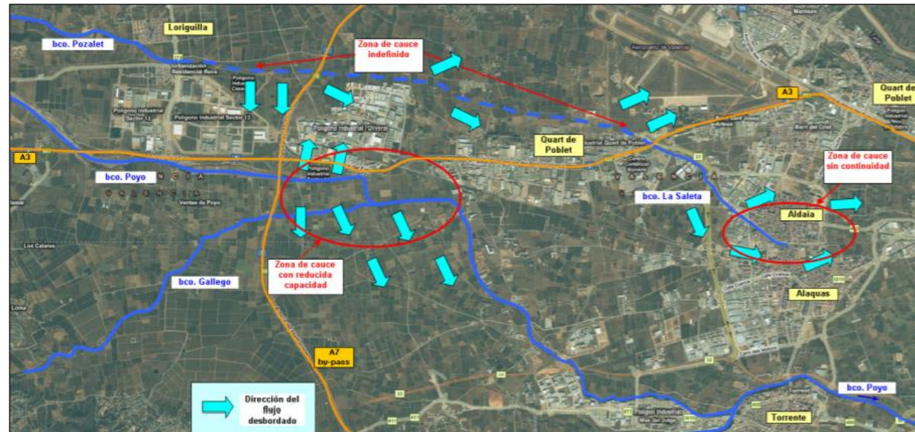
Figure 6. Hydraulic behaviour of the Pozalet-Saletta ravine. Source: F.Franch et al., 2010
