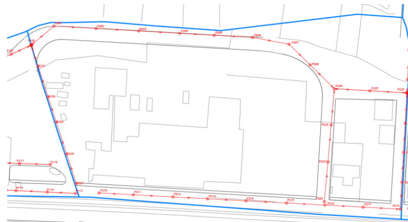
Figure 11. Collectors' design for catchment N2. Alternative 1
