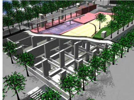
Figure 20. Example of an underground storm tank in an urban area. Source: MAGRAMA, 2014
