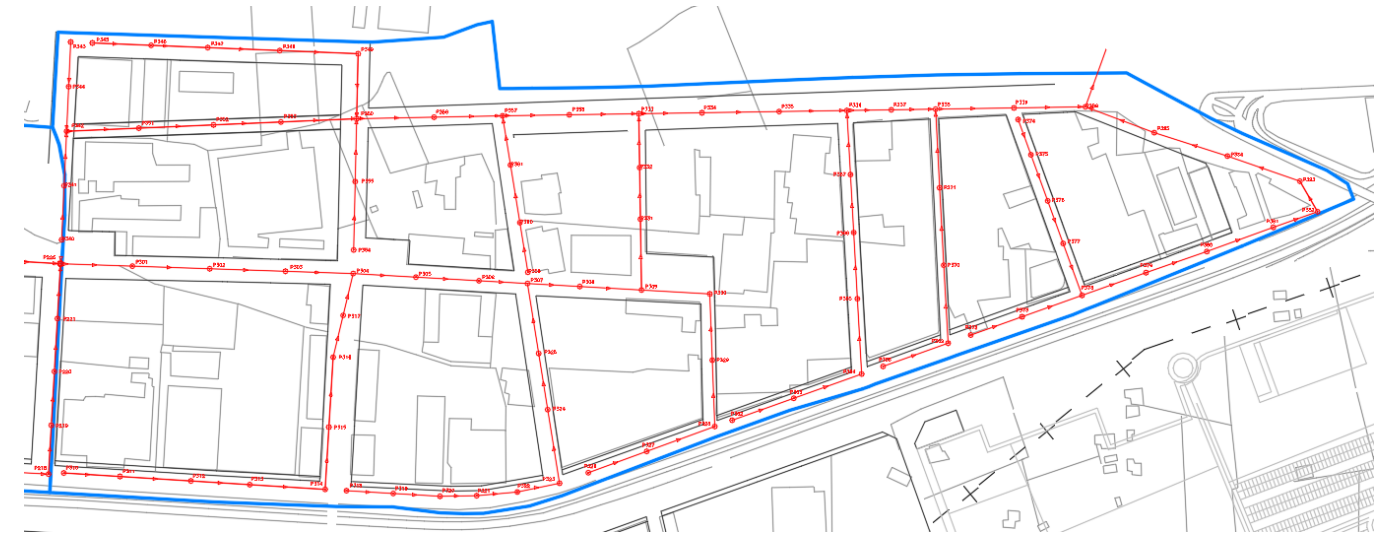
Figure 12. Collectors' design for catchment N3. Alternative 1
