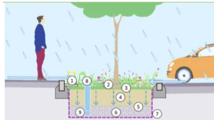
Figure 6. Rain garden scheme. Source: Perales, S. et al., 2019
