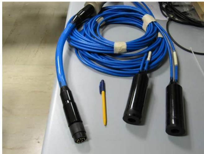
Figure 4.16: A picture of the two hydrophones (FFR-SX30 with SMID preamplifier) moulded by SEACON.
