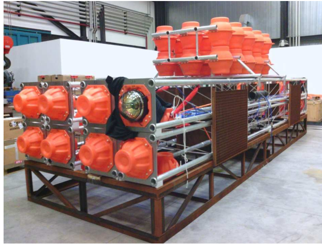
Figure 4.19: The NEMO-Phase II tower and the anchor.
