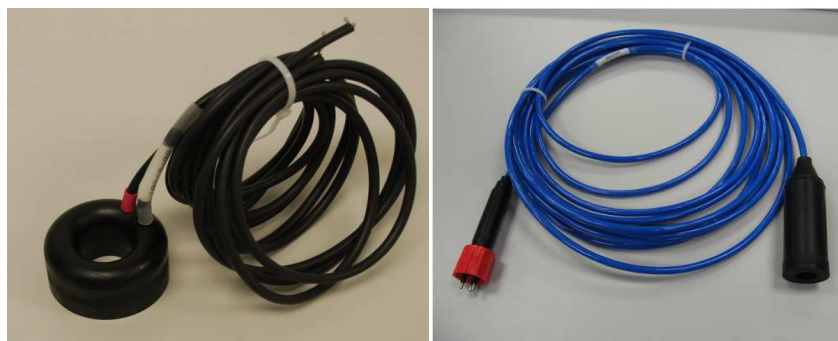
Figure 3.3: View of the Free Flooded Ring transducer with (right) and without (left) over-moulding.
