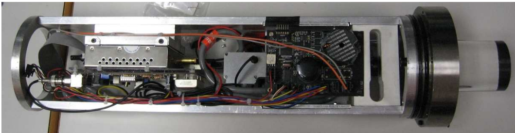
Figure 4.18: Inner view of the Laser Container. The laser and the integrated SEB can be seen.
