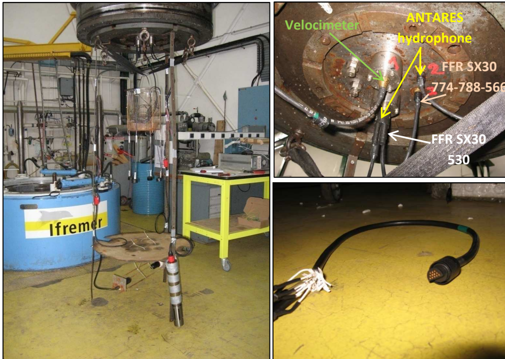
Figure 3.17: Views of the assemblage and the electrical connections used for the measurement (left and top right) and of the special connectors watertight up to 600 bars (bottom right).
