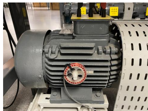
Fig. 5 Second tested motor (motor 2): 7.5 kW, 2 pole pairs
