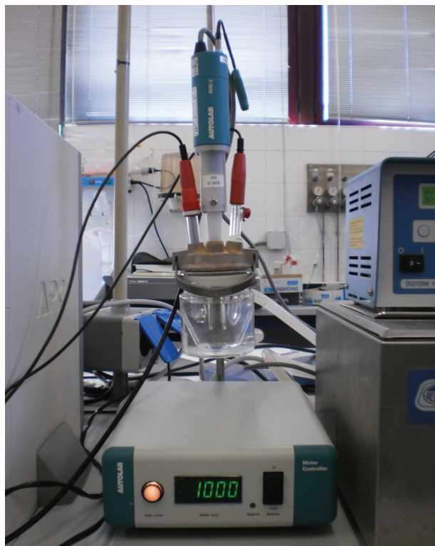
Figure 5.17. Experimental set-up with the working electrode mounted in a rotating disk electrode (RDE).
