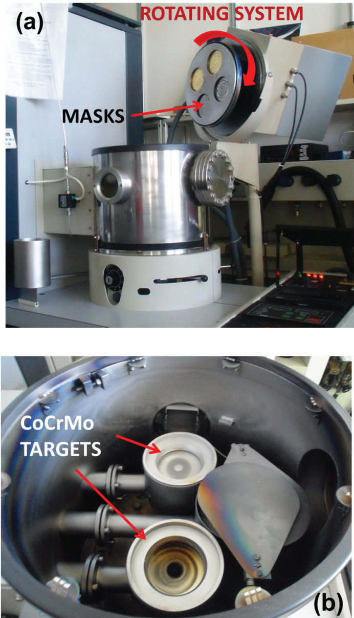
Figure 6.2. Magnetron Edwards ESM 100 PVD chamber with a (a) rotating part (top) and (b) the containers where the CoCrMo target is placed (bottom).
