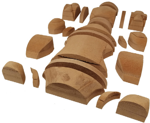
Fig. 13. Palazzo Mazzonis atrium MDF physical model of the vaulted system aimed to tactile experience of the vault (Source:own's, Digital fabrication by F. Ronco).
