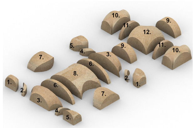
Fig. 12. Palazzo Mazzonis atrium 3D model (Rhinoceros®): different puzzle pieces (Source: own's. Modelling by F. Ronco).
