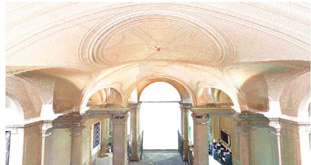
Fig. 6. Point cloud of Palazzo Mazzonis atrium. (Source: scan by M. C. López González; processing by F. Natta).
