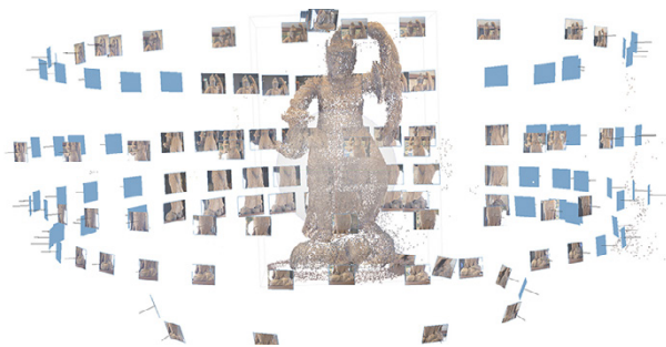
Fig. 5. Photo alignment with sparse cloud in Agisoft Metashape® software (photos: F. Ronco, S. Tamantini).
