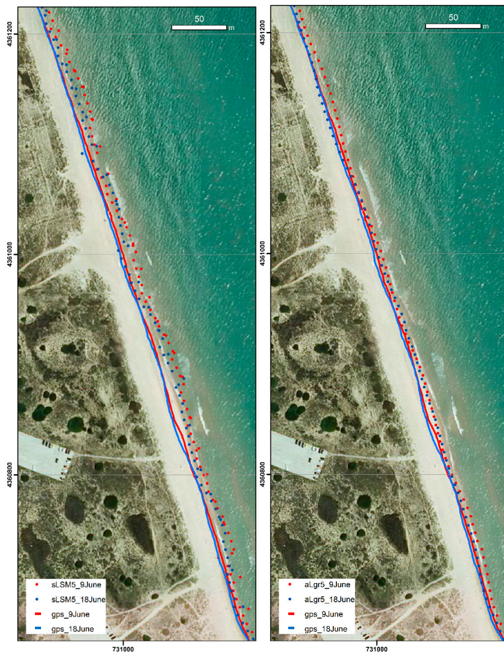
Figure 12. Coastal segment of El Saler beach where different shoreline solutions are shown for 9 and 18 June in red and blue respectively. The GPS shorelines are represented with lines and the sub-pixel shoreline solutions with dots (sLSM5 and the aLgr5). Solutions painted on an orthophoto taken from 2015 PNOA sources. The grid coordinates are GCS_ETRS89 UTM30N.
