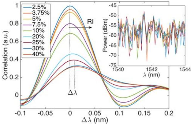
Fig. 7. Mutual correlation (normalized between to a value of 1) between the reference signature (in water) and the signatures acquired at different levels of sucrose (2.5% to 40%) for sensor RI1. The inset shows a portion of the signatures, reporting the power as a function of wavelength.
