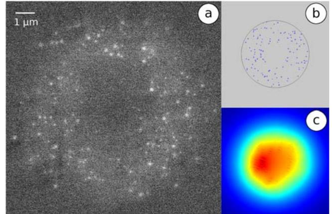
Fig. 1. (a) SEM of the NP-doped fiber cross-section; (b) schematic of the cross-section realization used for the simulation; (c) Modulus of the FM magnetic field.
