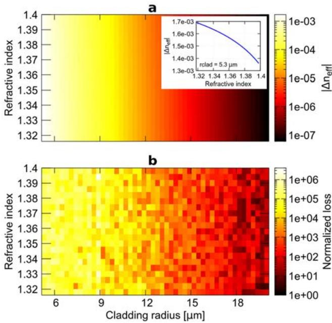
Fig. 2. FEM based simulation of the etched MgO-NP fiber, varying the radius of the cladding and the refractive index of the external solution to analyse. Colour maps of: (a) the differential effective index of the FM with respect to the unetched fiber; (b) the propagation loss of the FM, normalized to the loss of the unetched fiber.
