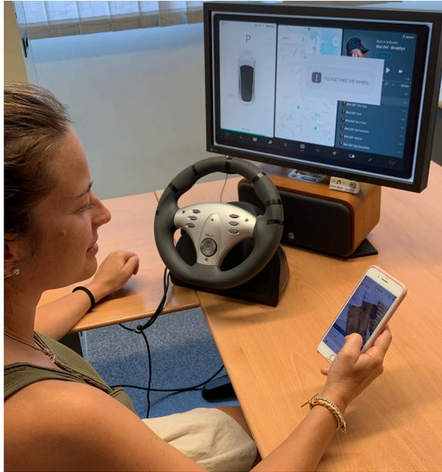
Figure 9: Scenario of the Supervised Autonomous Driving task with an inattentive driver
