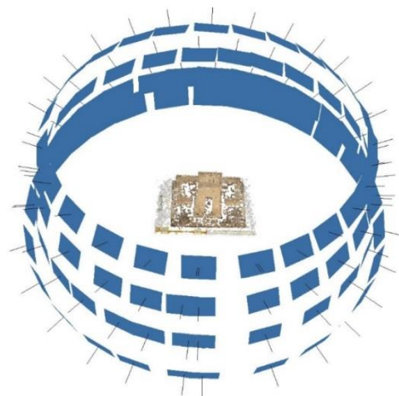
Figure 5: Image orientation and extraction of a sparse cloud of tie-points.
