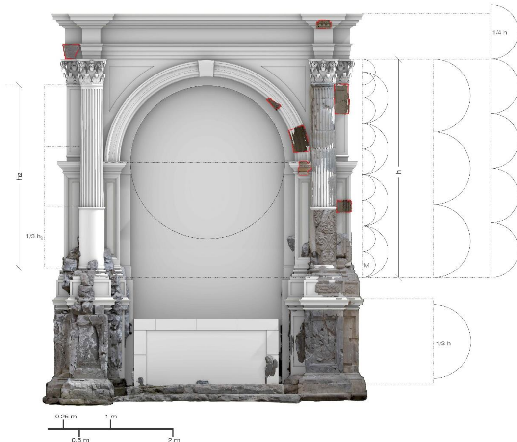
Figure 13: 3D model of the altar of Madonna del Carmelo. In white, NURBS. In the original colours, photogrammetric mesh of the surviving parts. In red, virtual anastylosis.
