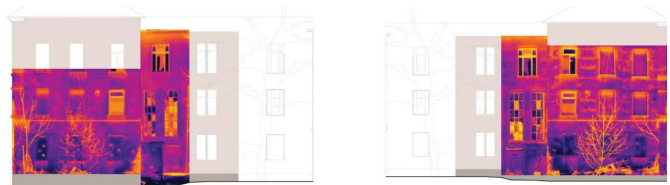
Fig. 13: North façade -time: 11:00 and 15:00
