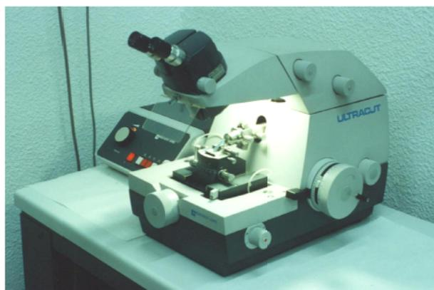
Figura III.3.3. Ultramicrotomo Ultracut de Reichert-Jung.
