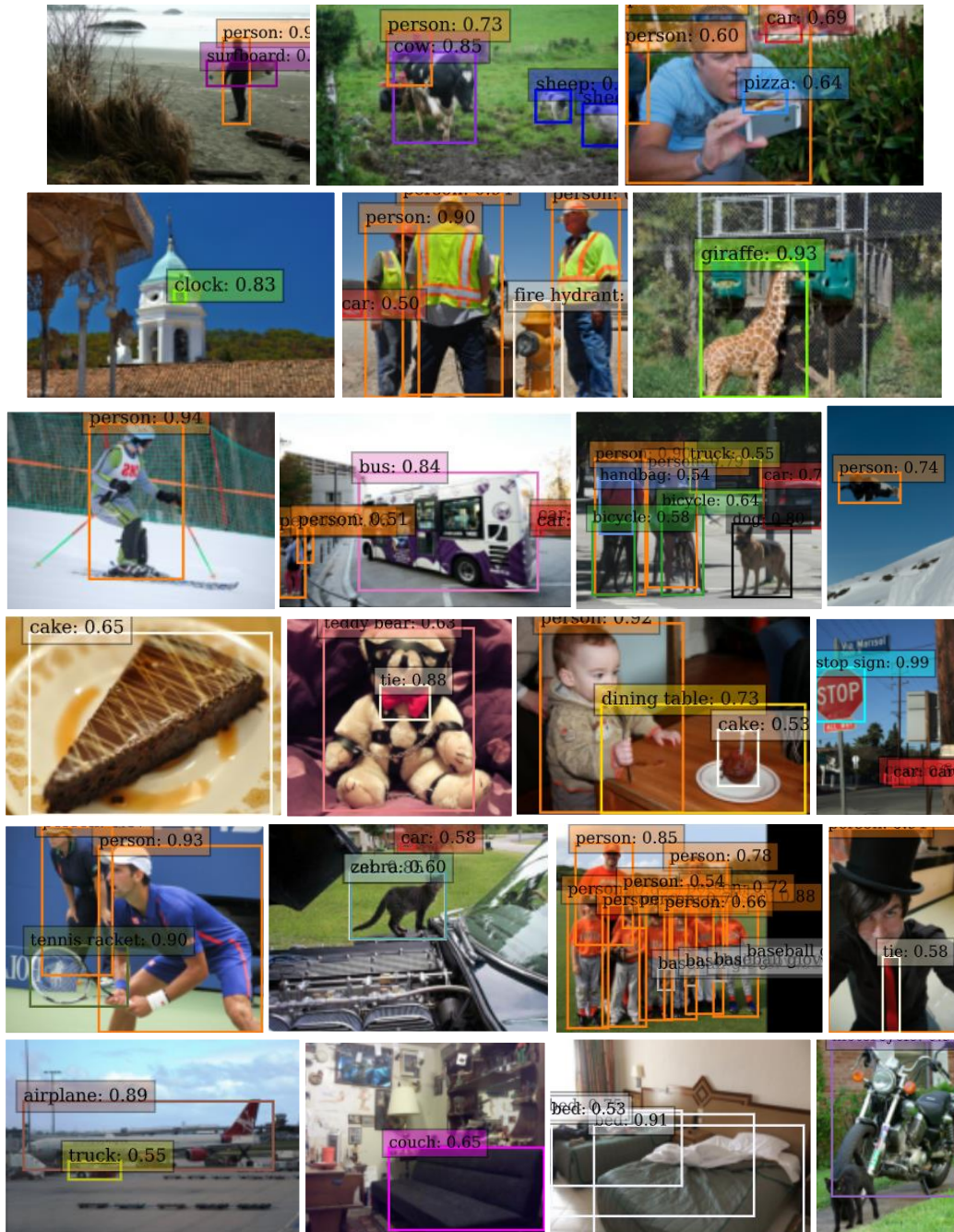
Figure A.2: Object detections performed by the spiking-RetinaNet model with a 2s integration time-window and disregarding of the transient. Images belongs to the MS COCO dataset [48].
