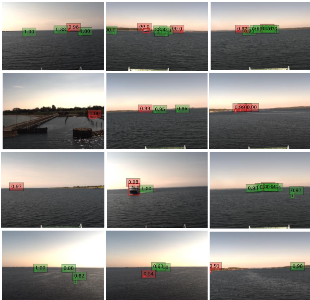
Figure A.1: Object detections performed by the spiking-RetinaNet model with a 1s integration time-window and disregarding of the transient. Boats are framed red and buoys green. Images belongs to the ShippingLab dataset.
