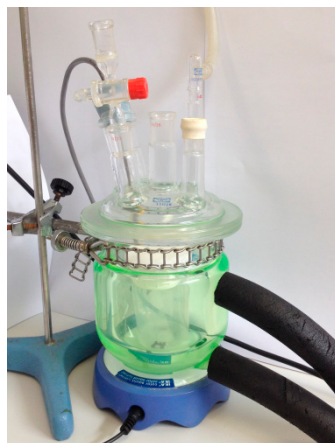
Figure 4. Thermostated cell for conductivity tests in solutions.
