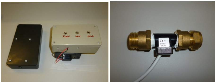
Figure 24 Hot water flow meter
