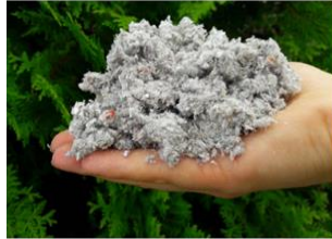
Figure 1: Loose fill cellulose insulation material
