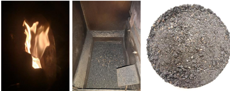
Figure 4.25. Flame during combustion (left), residue into the incineration unit after combustion (middle), and collected ash (right).
