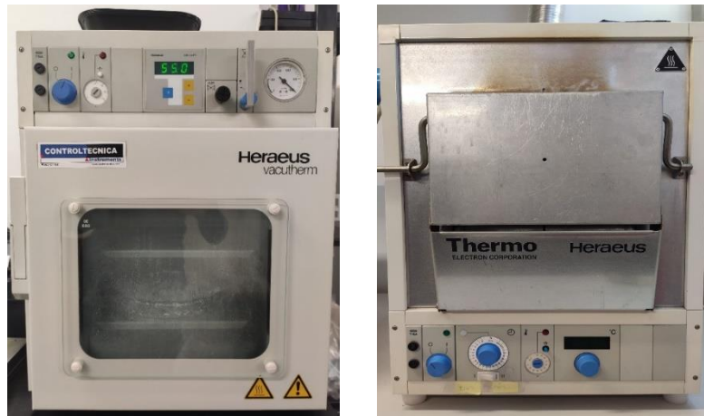
Figure 3.1. Vacuum oven (left) and muffle furnace (right) used in proximate analysis.
