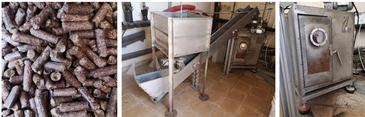
Figure 3.7. Pellets of beer spent grains (BSG) and incineration pilot plant.
