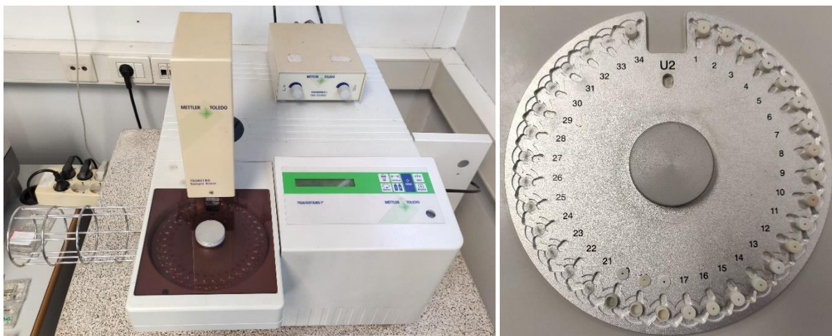
Figure 3.4. (a) Mettler-Toledo TGA 851 series and (b) 70 \mu\text{L} alumina capsules containing ash.
