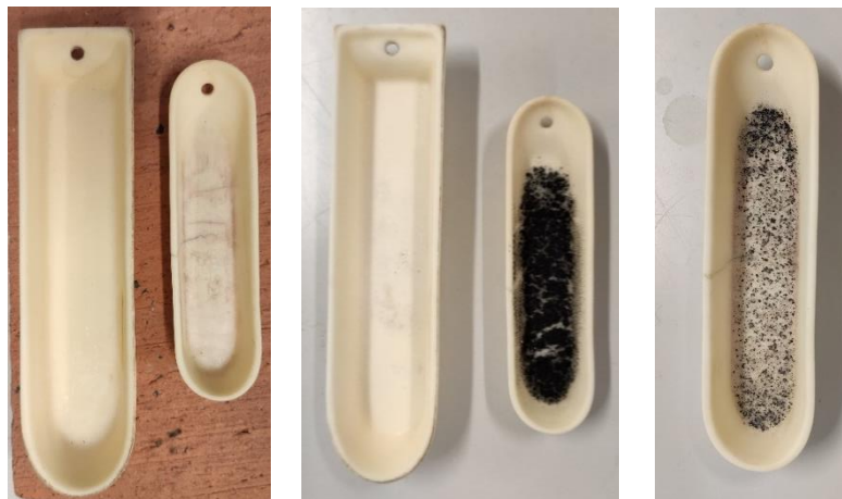
Figure 3.2. Alumina pan (a), residues of volatile matter (b) and residues after the experiment for the determination of ash (c).
