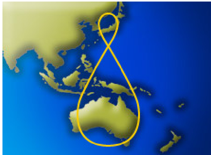
Figure 21. Analemma pattern followed by the three geosynchronous satellites of the QZSS constellation [10]
