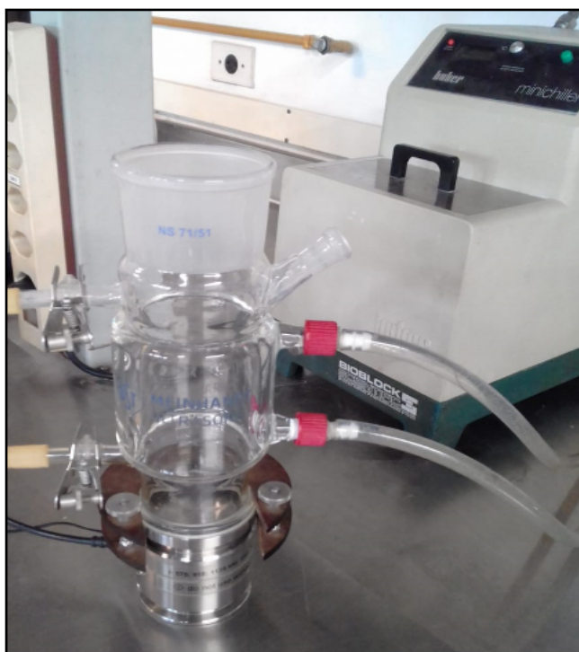
Figure 17: US reactor with cooling jacketed, with permission of E. Serna-Galvis
