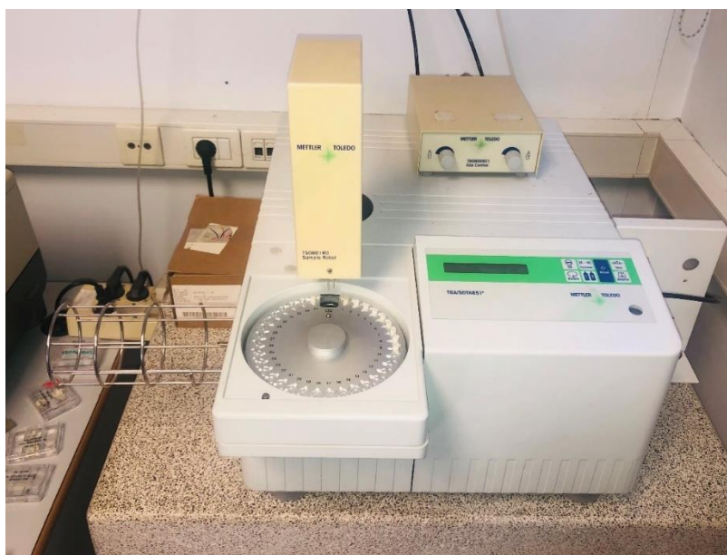
Figure 3.2: Mettler-Toledo TGA 851 series with 70 \mu\text{L} alumina capsules containing ash.
