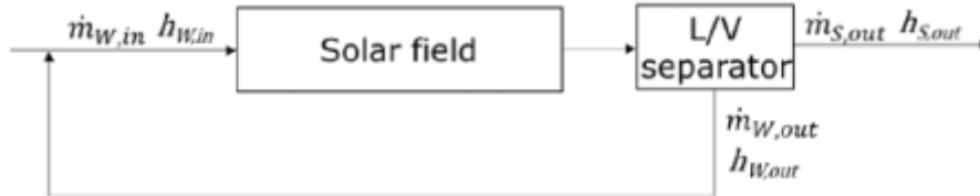
Figure 27. Direct steam production with a solar field [33].
