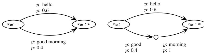
**Figure 1.8:** Example of conversion of a phrase graph (left) into a word graph (right).
