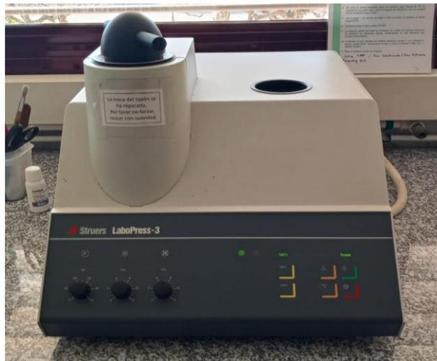
**Figura 14.** Embutidora LaboPress-3 de Struers.
