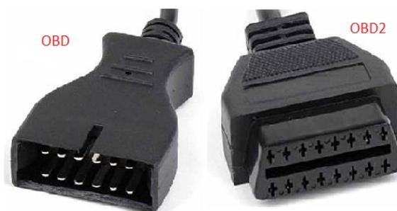
Figura 6: Comparativa conector OBD vs OBD2
