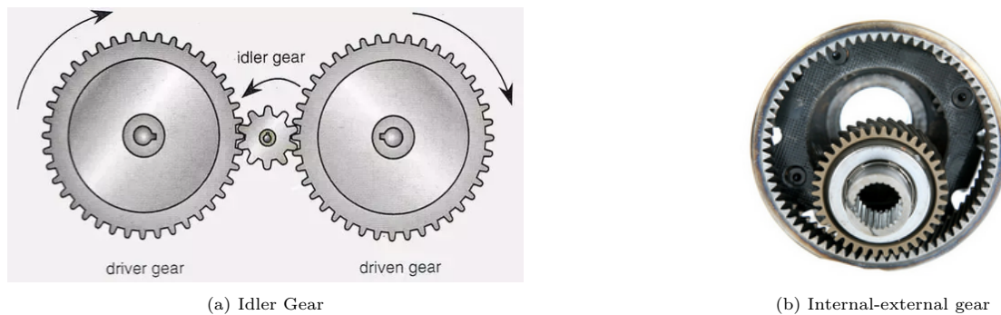
Figure 63: Gear teeth Placement
