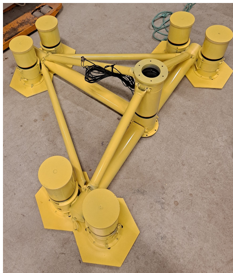
Figure 4.4: The lab-scale TetraSub floater designed and manufactured by SOT.
