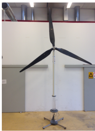
(b) The 1:60 TLP floating wind turbine model for the 2015 experimental campaign at DHI.
