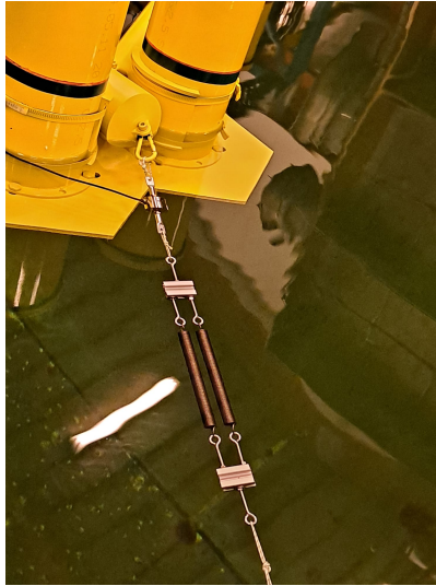
Figure 4.14: Force mooring gauge with the previous mooring line system.
