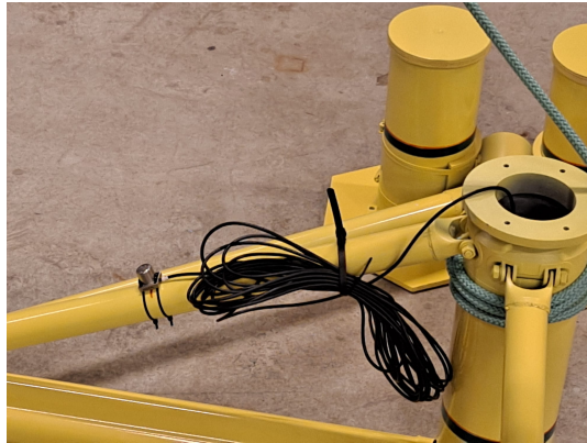
Figure 4.15: Analog accelerometer mounted on the front brace of the floater.
